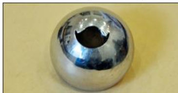
Figure: Metal hip prosthesis causing cobalt intoxication. Severely damaged metal head with hole due to severe metal ion.
